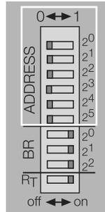
Figure 25: DIP-switches on the gateway
