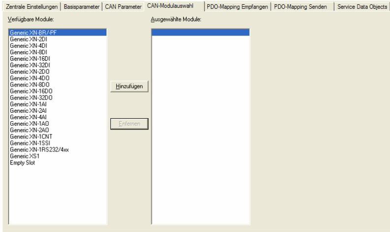
Figure 37: CAN module selection of the CAN slave (in this case: XN-GWBR-CANopen)
