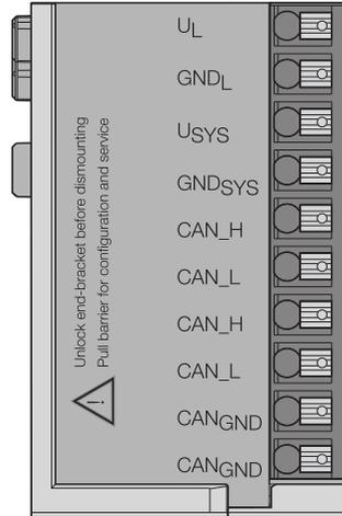
Figure 21: Push-in tension clamp terminals at XNE-GWBR-CANopen
