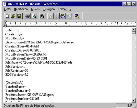
Figure 29: Header of an EDS file for XI/ON
