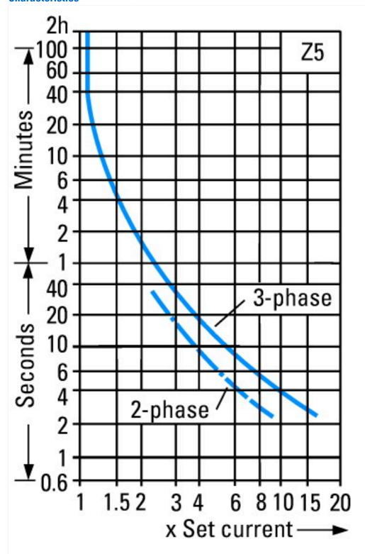
These tripping characteristics are mean values of the spreads at 20 °C ambient air temperature in a cold state.
