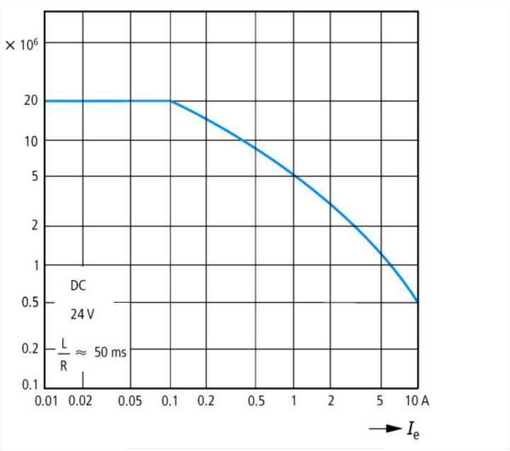
$$\label{eq:component lifespan (operations)} \begin{split} & l_e = \text{rated operational current} \\ & \text{Three contacts in series} \end{split}$$
