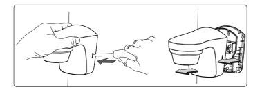
➤ Using the screwdriver, carefully loosen the snap-in hook at the side and pull the device forward.
