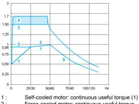
2: Force-cooled motor: continuous useful torque
