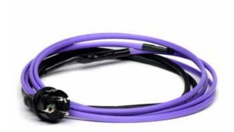
**PipeHeat-10** is a self-regulating heating cable with a plug, of **10 W/m** output, and Adflex (polyolefin) overjacket. **PipeHeat-10** can be installed directly on a pipe's surface or inserted into pipe through a metal fitting otherwise.
