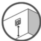
Place the thermostat at a suitable height on the wall (typically 80–170 cm). Switch can be placed on free area on the wall.
