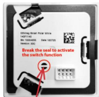
A “room only” option is also available, but requires that you have to break the small plastic seal and the seal in the print board below, on the back of the display module, e.g. using a screwdriver; reset is needed; it will be possible to set the
