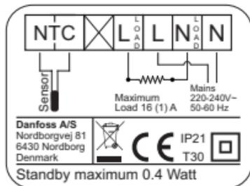
**Note:** Always install the floor sensor in a conduit in the floor.
