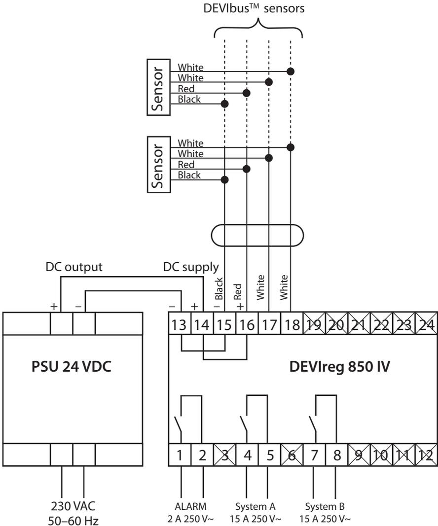
The DEVIreg™ 850 has an integral alarm function that monitors the attached sensors and the in-built microprocessor. An external alarm may also be connected to the system.
