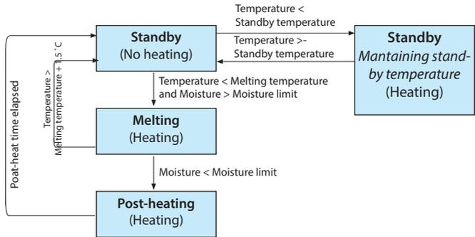
Hence it is known whether heating of the ground area is needed in order to avoid that the ground area is covered by ice and snow.
