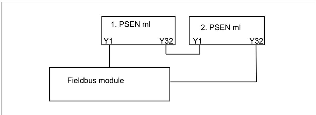
► Series connection of the solenoid operation
