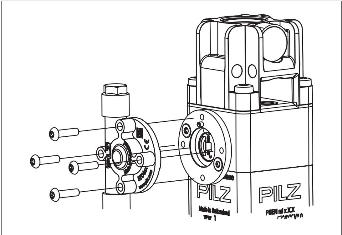
4. Screw the housing of the escape release with the screws [1] to a mounting surface with 6 - 6,5 Nm (see diagram).
