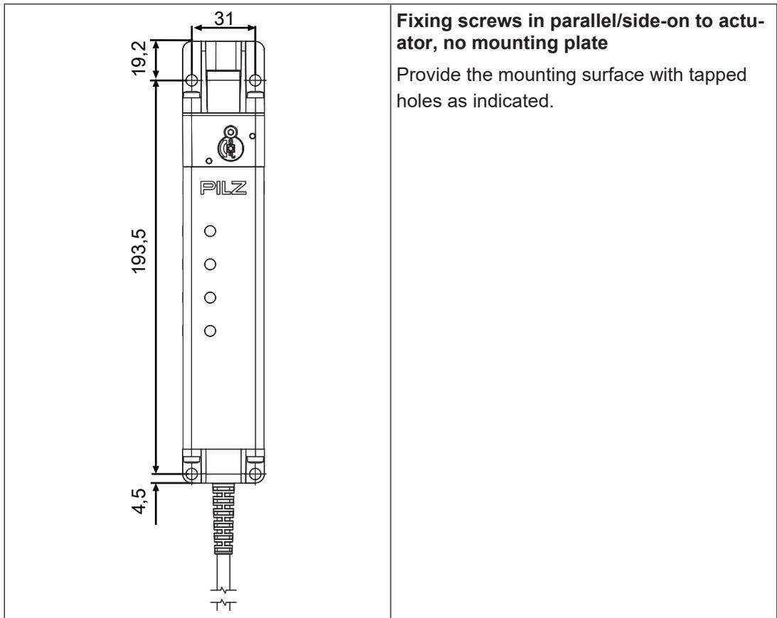
**Fixing screws in parallel/side-on to actuator, no mounting plate**
