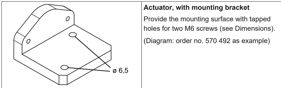
1. Use two M6 screws to fix the mounting bracket to the gate. The position of the drill holes can be taken from the section entitled Dimensions.
