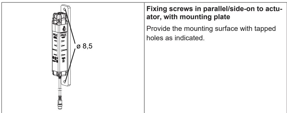
**Fixing screws in parallel/side-on to actuator, with mounting plate**
