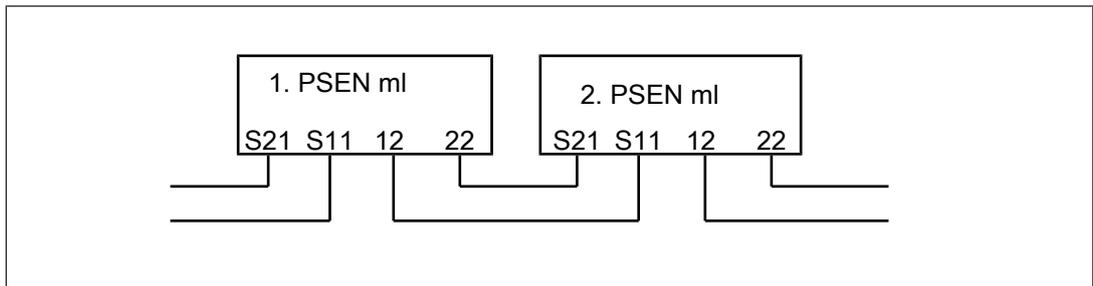
► Series connection of diagnostics with Safety Device Diagnostics
