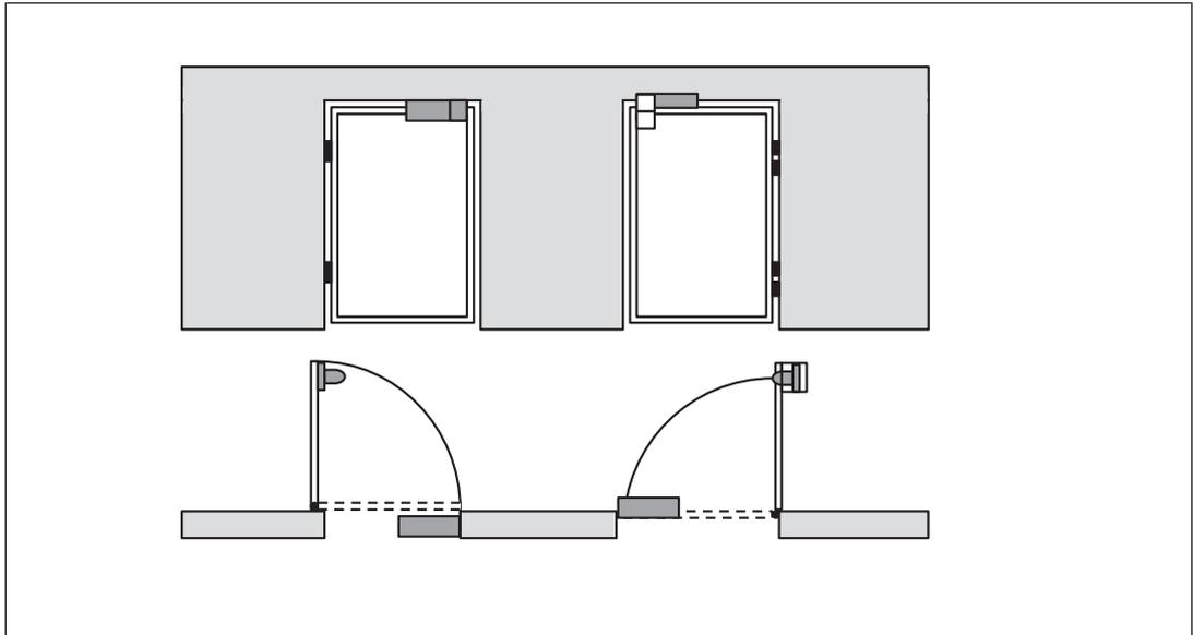
Maintain a slight shift of the rotation point of the door when installing the actuator.
