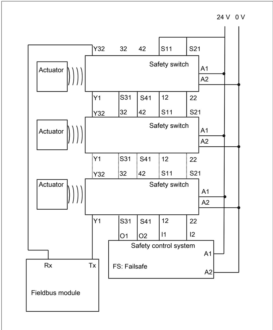
For connecting the safety switch PSEN ml sa 1.1/2.1/2.2 in a series connection there are the following options:
