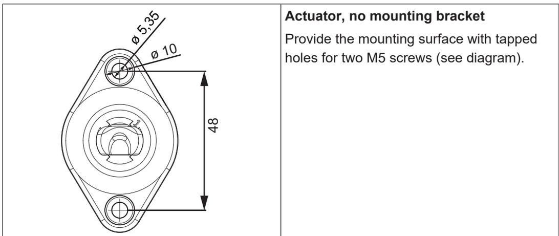
1. Attach the actuator to the gate.
