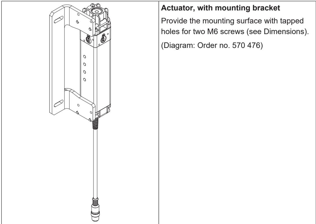
1. Use two M6 screws to fix the mounting bracket to the gate. The position of the drill holes can be taken from the section entitled Dimensions.
