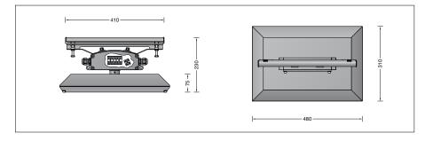
Lamp Module connected wattage 62 W Luminaire connected wattage 69 W
