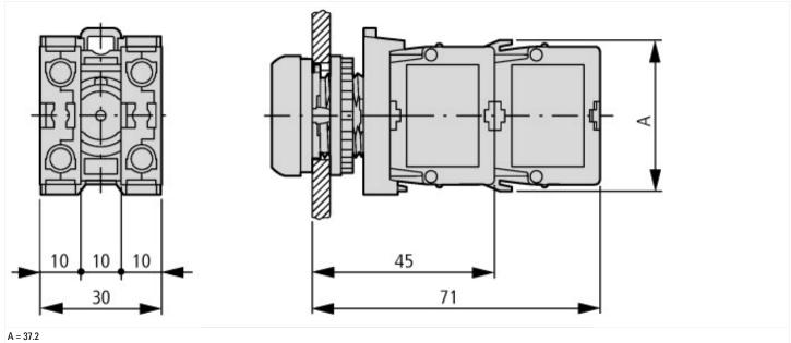
Pushbutton with M22-(C)K... Pushbutton with M22-(C) LED... + M22-XLED...
